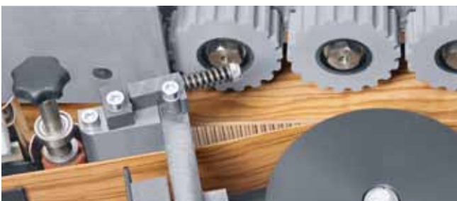
Edging with thick edge on a standard edging machine.
