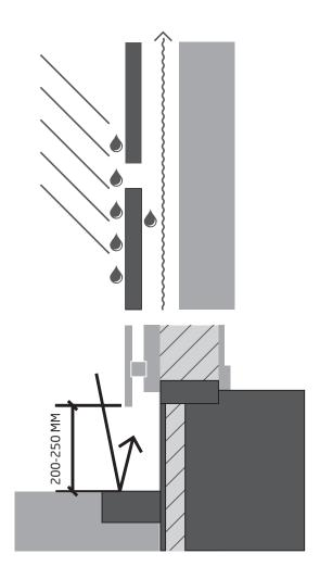
Note that panels should be fitted with spacers and not fitted flush to any masonry or brickwork.
